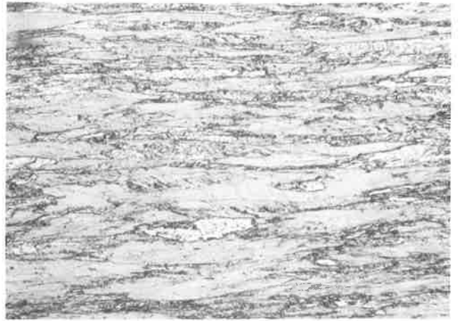
BSD Tungsten swaged rod 4 mm \varnothing Magnification approx. 45x
